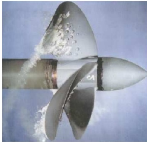
Fig – Cloud cavitation on hydrofoil (left) - Bubble cavitation on propeller (right) [Franc and Michel, 1995]
